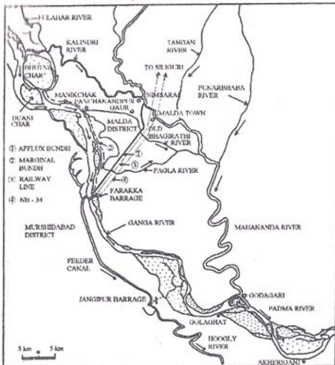
Fig. 3 River Ganga and its tributaries near Malda Town showing meandering near Farakka Barrage.
