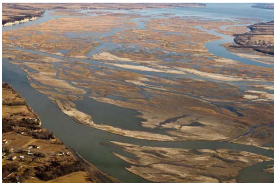
Fig. 4 : Sediment Deposition in Reservoir Behind Gavins Point Dam on the Missouri River
