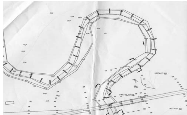
Fig. 10 Formation of a Bowl upstream and downstream of a ridge (on M.P. State Highway) due to excessive restriction of waterway
