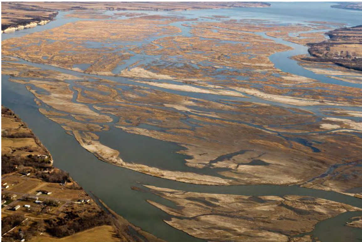
Fig. 9 Sediment Deposit in Lewis and Clark Lake - reservoir created by Gavins Point Dam on the Missouri River. It's 30 percent full of sediment and could be half full by 2045
